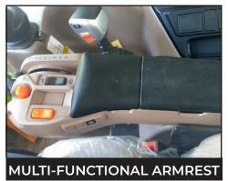
The multi-functional electronic armrest allows numerous functions like throttle engagement, 3 point linkage lift and lower, Powershift and Auto Powershift mode.
