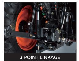
The electronic controlled 3 point linkage system boasts a 4852kg lifting capacity allowing for the installation of a variety of working implements.
