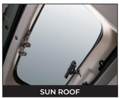
A transparent sunroof inside the cabin ensures an upward clear vision when using the loader, improving ease of operation and safety.
