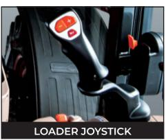
The multi-functional loader joystick is built with 3rd service and Powershift buttons making for easy loader working conditions for the user.
