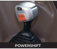
A simple button operation on the side speed lever and armrest gives you a 32x32 transmission with an 8-speed Powershift in 4 ranges.
