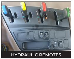
Changing or removing implements is light work thanks to the four external rear hydraulic ports and one-handed quick couplers with a flow at the remotes of 118 lpm.
